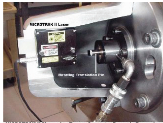
MICROTRAK II Measuring Torque Converter Dynamic Expansion
