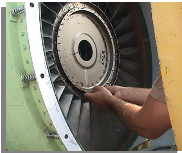
Knowing exactly where to install weights eliminates errors
