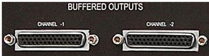
**Buffered Odd Tooth TTL Outputs** – Two additional TTL level 1/revolution outputs for test cell instrumentation.
