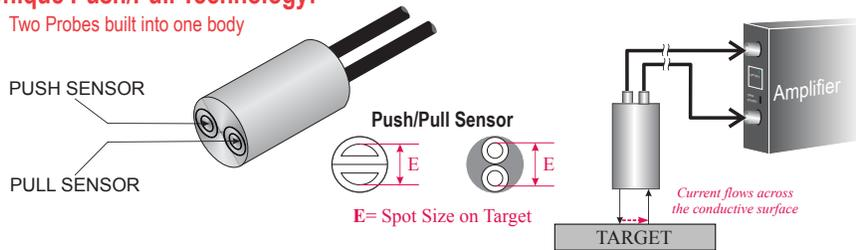
The Push-Pull probe is a unique version of MTI's Accumeasure™ amplifier series. This special design provides accurate surface information for wafer bow and warp.
