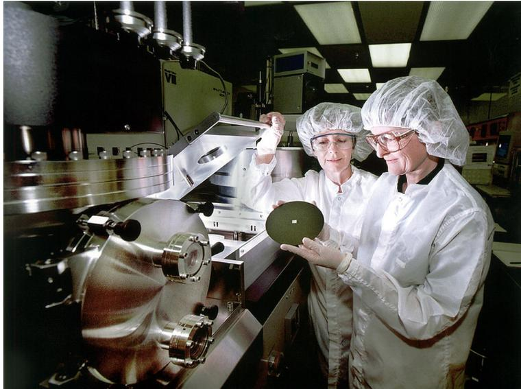
Semiconductor wafers such as those used to make integrated circuits (ICs) and silicon photovoltaic (PV) cells are fragile and expensive. The ability to precisely measure critical wafer parameters such as bow and warp not only ensures the integrity of circuit patterns, it improves yields and lowers production costs.
