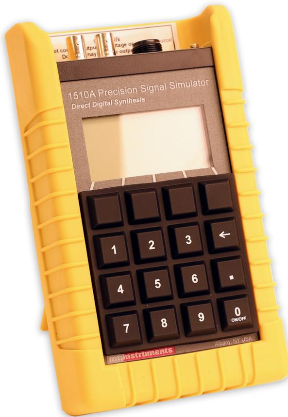
*MTI's 1510A Portable signal generator can reproduce the specialized N1 and N2 speed signals generated by gas turbine engines, distinguishing between multiple teeth of same height and the one odd tooth.*
